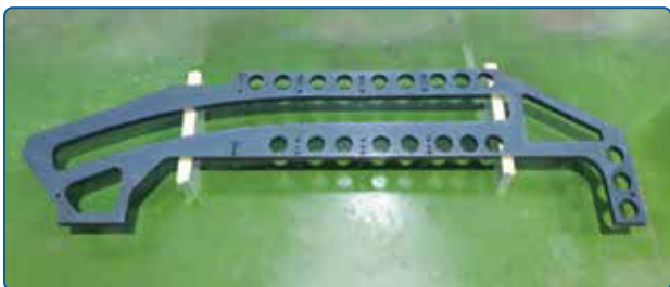
SCM440-16*460*1610 Heat Treatment 28-32HRC Nitriding Treatment 700H v depth 0.1 熱処理HRC28~32、窒化処理Hv700深さ0.1
